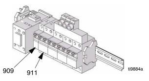
FIG. 10: Circuit Breaker Module
