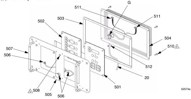
Detail of Membrane Switches and Display Boards
