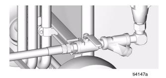
Turn both PRESSURE RELIEF/SPRAY valves (SA, SB) to PRESSURE RELIEF. Route fluid to waste containers or supply tanks. Ensure gauges drop to 0.
