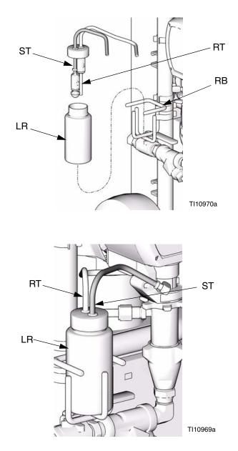
FIG. 13. Pump Lubrication System
